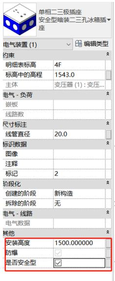
The screenshot shows a software interface for configuring an electrical device. The title bar indicates '单相三极插座' (Single-phase three-pole socket) and '安全型暗装二三孔冰箱插座' (Safety type recessed two-hole three-hole refrigerator socket). The '其他' (Other) section is highlighted with a red box, showing the following parameters:
