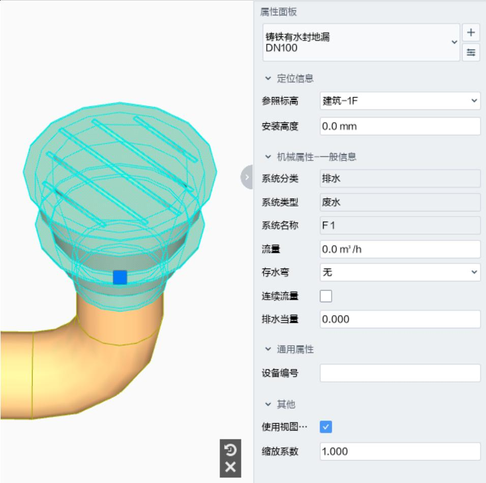
The screenshot displays a 3D model of a cast iron water seal floor drain on the left, rendered in a semi-transparent cyan mesh. To its right is a vertical property panel titled '属性面板' (Property Panel). The panel is organized into several sections:
