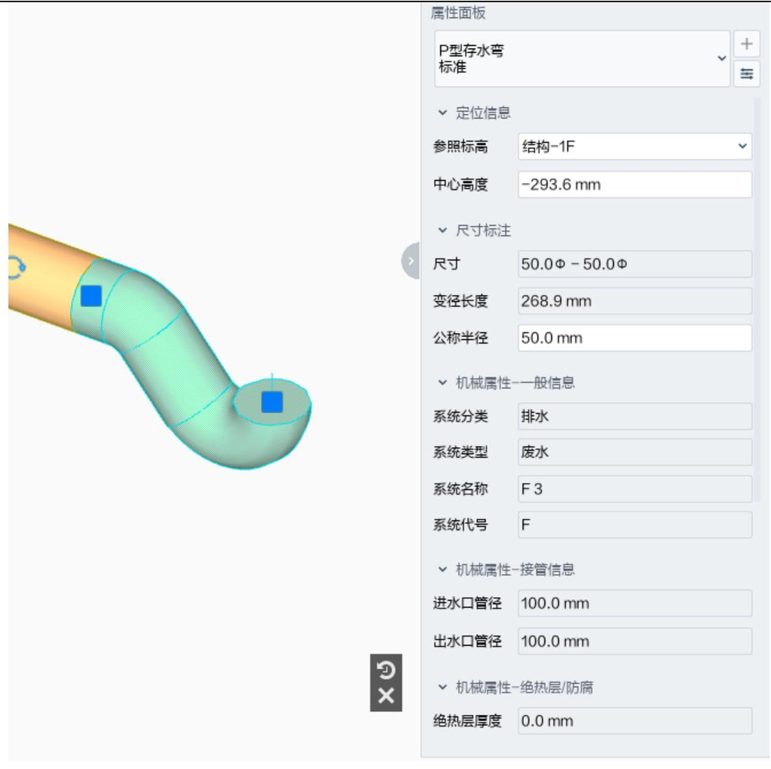
The image shows a 3D model of a P-type water trap (P型存水弯) in a light blue color. The trap is connected to a horizontal pipe on the left. The property panel on the right contains the following information:
